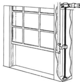
Automatic switch on large windows (doors)
